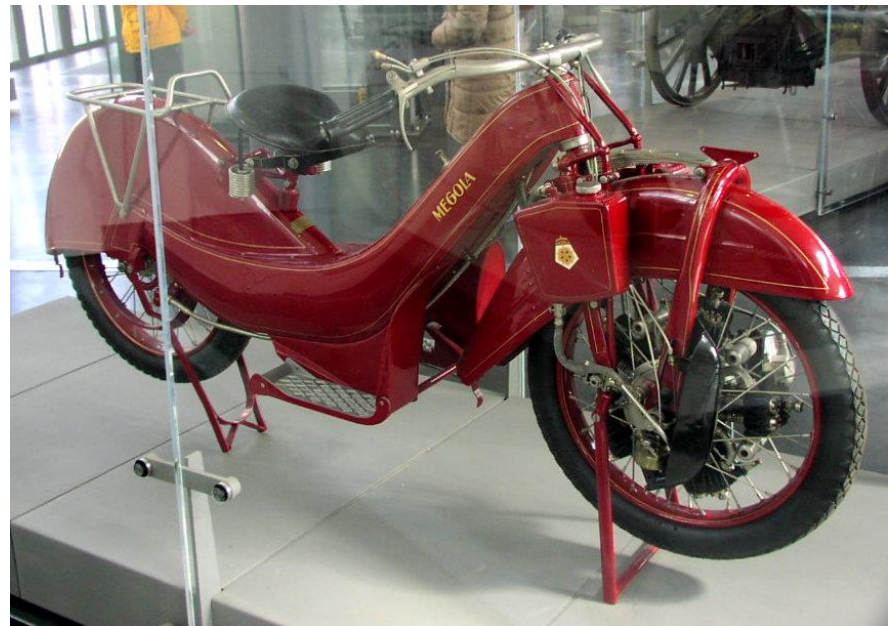
Megola motorcycle with rotary engine mounted in the front wheel
